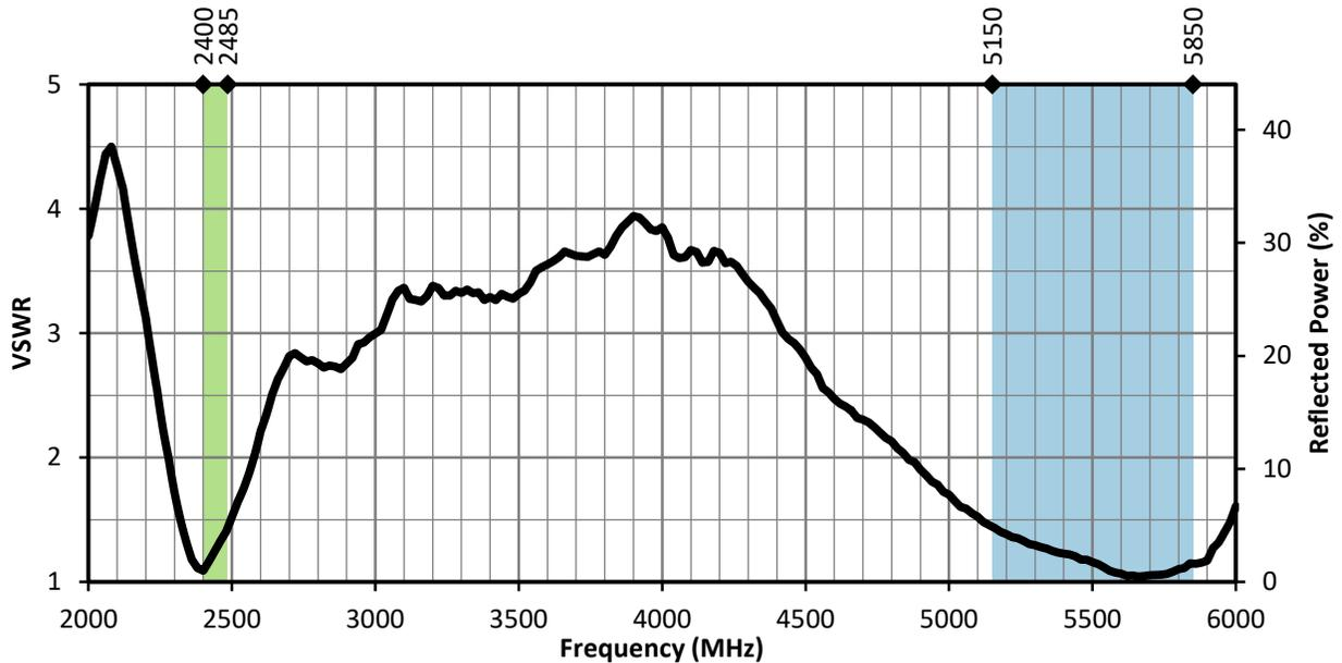
Figure 3. LPD VSWR, Bent-90, with Frequency Band Highlights
