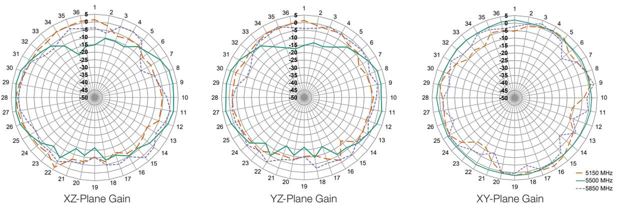
Figure 15. Radiation Patterns for LPD, Straight
