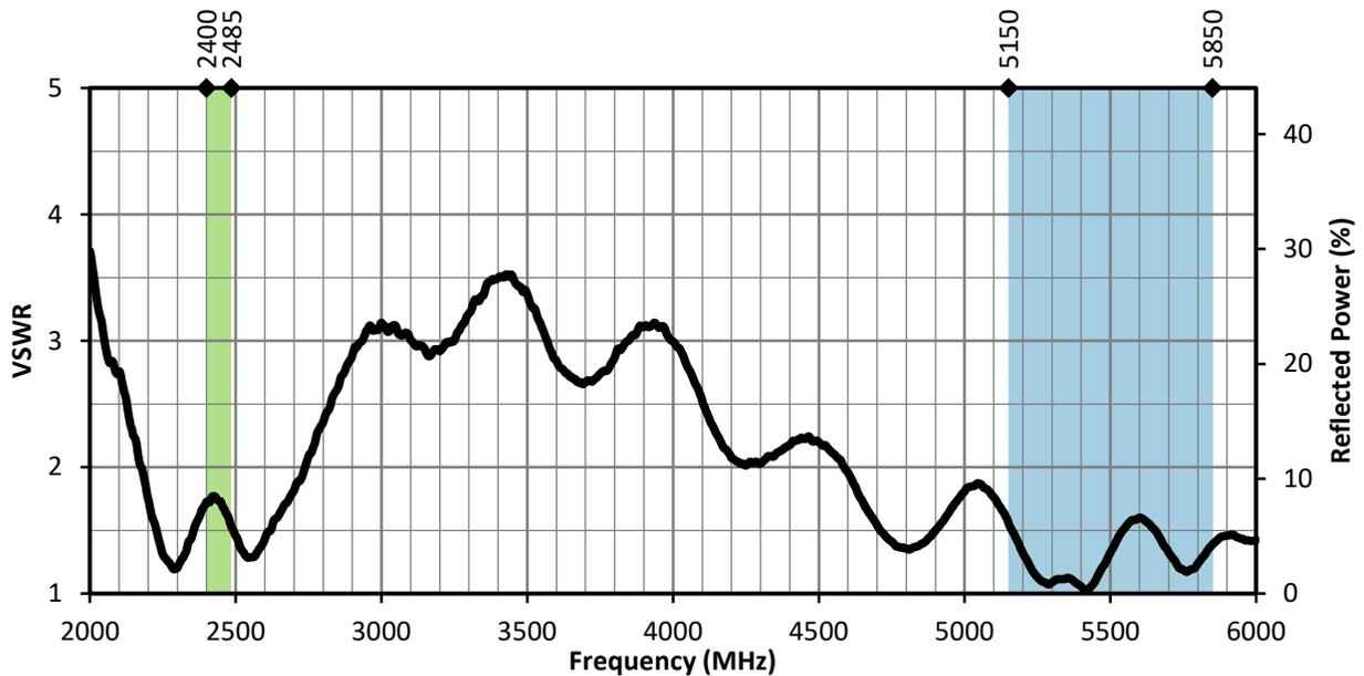
Figure 10. LPD VSWR, Straight, with Frequency Band Highlights
