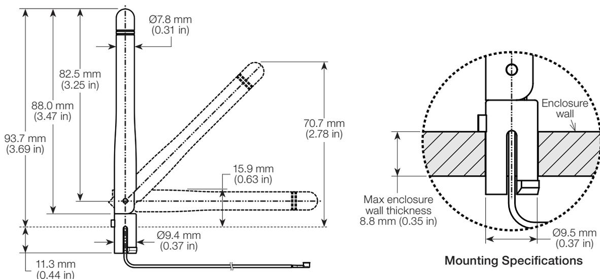
Figure 1. ANT-DB1-LPD-125 Dimensions and Mounting Data
