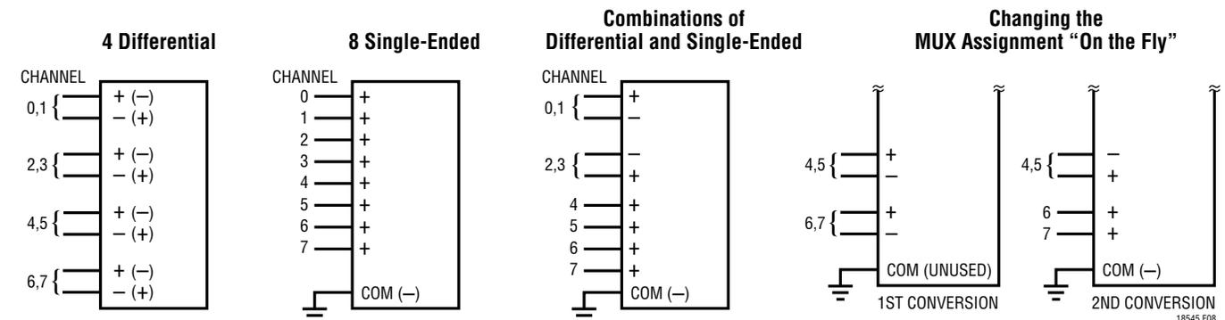
Figure 8. Examples of Multiplexer Options on the LTC1854/LTC1855/LTC1856
