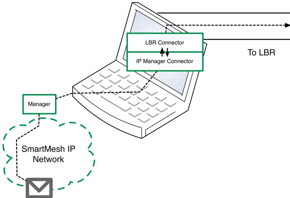
The LBR client is a computer program running on the computer physically connected to the SmartMesh IP Manager. It consists of these components:
