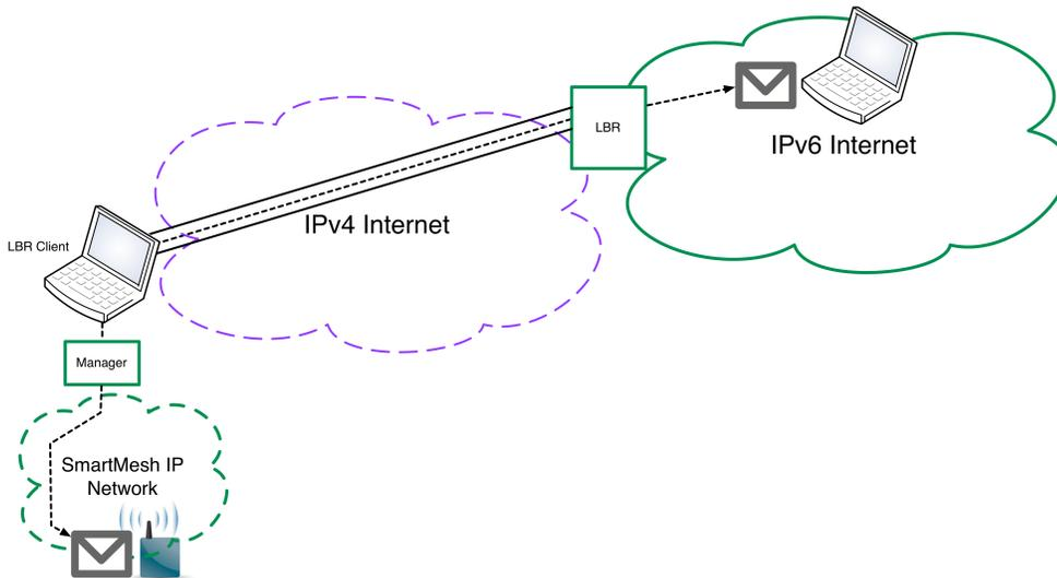
Once your SmartMesh IP Manager is connected to the LBR, the IPv6 packets exchanged between the SmartMesh IP network at the IPv6 internet are "tunneled" through the connection between the SmartMesh IP Manager and the LBR.
