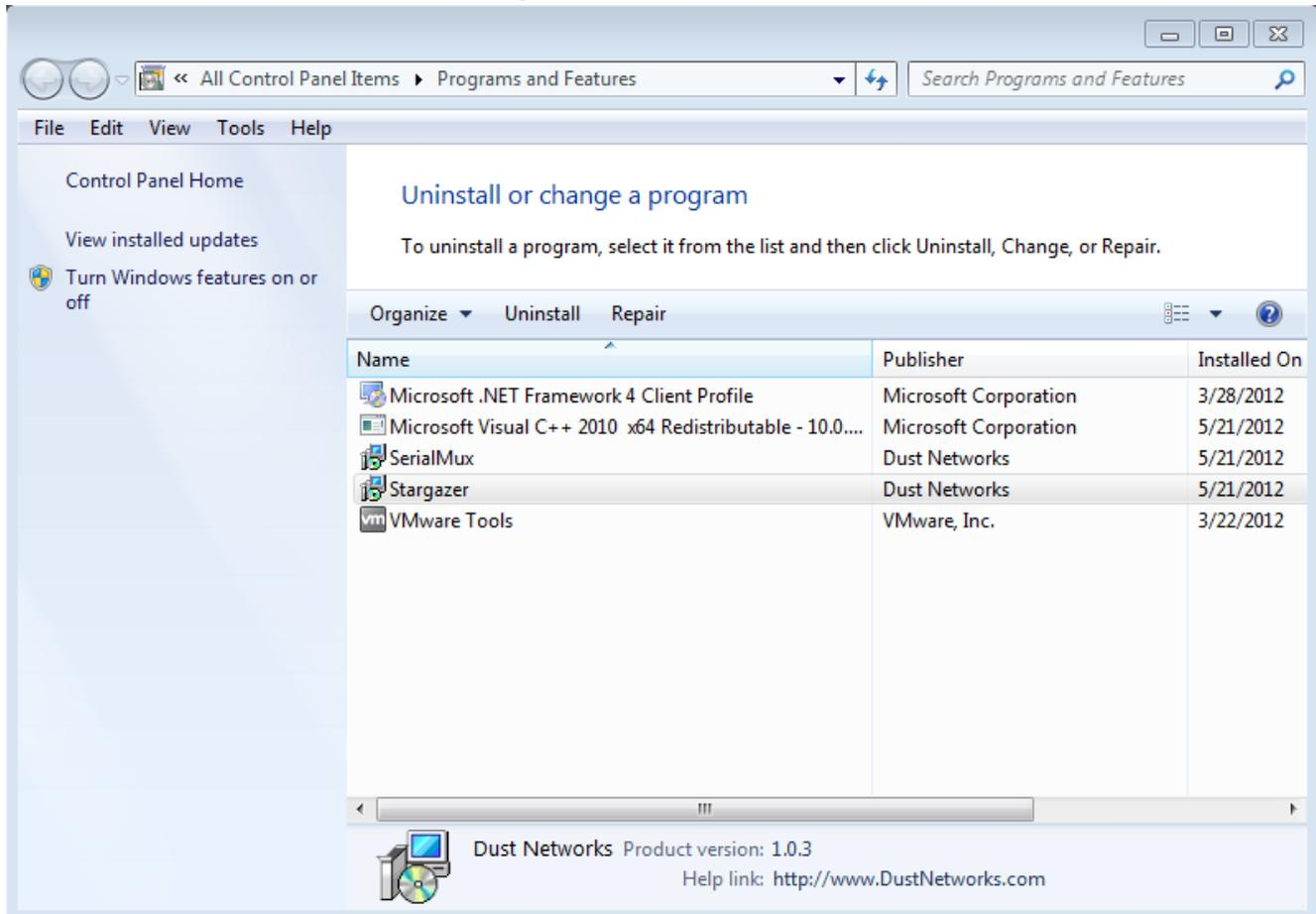
Select **Stargazer** (or the tool that you are upgrading) from the list, right click and select **Uninstall**. Any dependencies that were installed, such as the .NET Client Framework, do not need to be removed unless the installation instructions indicate otherwise.
