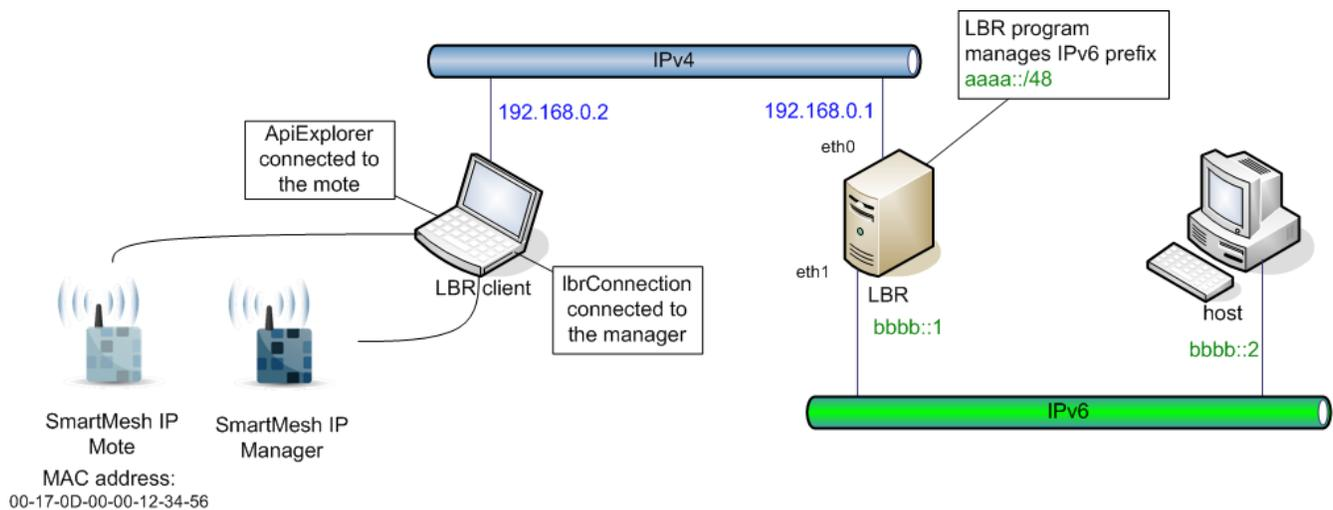
The diagram above represents the connections and the addressing used for these installation steps. Replace the addresses with the ones applicable to your situation.
