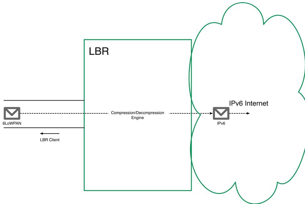
To increase efficiency, the 6LoWPAN protocol is used inside the SmartMesh IP network, a compressed version of IPv6 protocol. The LBR contains a compression/decompression engine which turns 6LoWPAN into IPv6 on-the-fly as data is exchanged between the SmartMesh IP network and the Internet.
