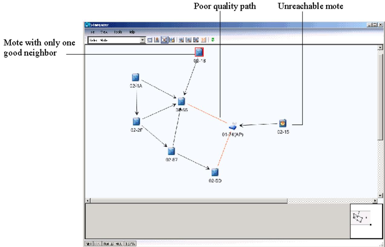
If connectivity problems persist for any mote after the network has been running for an hour, you can manually intervene by trying one of the following:
