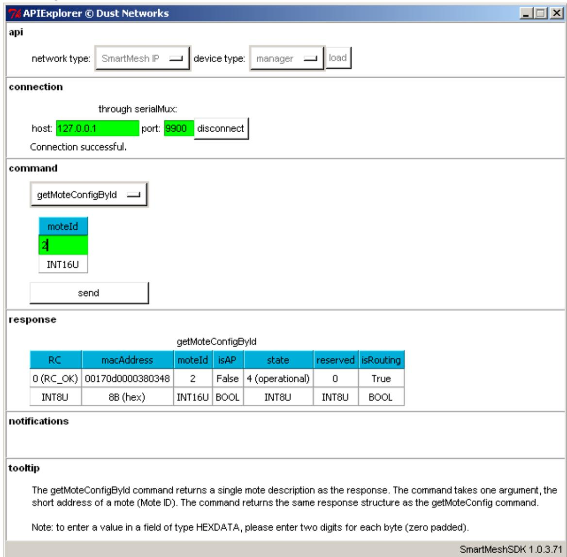
The screenshot shows the API Explorer interface for Dust Networks. The 'api' section has 'network type' set to 'SmartMesh IP' and 'device type' set to 'manager'. The 'connection' section shows a successful connection to host '127.0.0.1' on port '9900'. The 'command' section shows the command 'getMoteConfigById' with 'moteId' set to '2'. The 'response' section displays a table with the following data:
