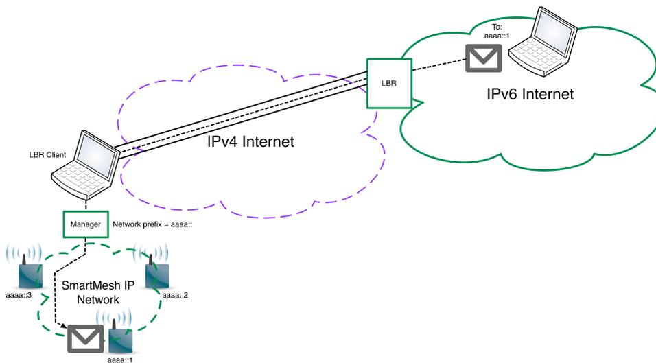
When running in server mode, the LBR manages a pool of IPv6 addresses, which it assigns to the different SmartMesh IP networks connecting to it. When a client connects to it, after authenticating the client, the LBR assigns it a network "prefix", i.e. the network part of the IPv6 address of each node in the SmartMesh IP network.
