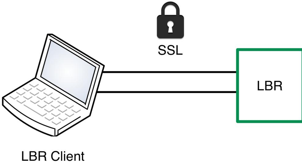
To enable confidentiality, data integrity and authentication, the session between the LBR client (connected to the SmartMesh IP Manager) and the LBR can be secured through a Secure Sockets Layer.
