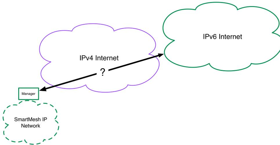
Today, there are two versions of the Internet: the older IPv4 version and the new IPv6 version. While a SmartMesh IP network is IPv6-ready, most of the current Internet still run on the older IPv4 version. The LBR understands both version, allowing for an SmartMesh IP Manager to connect to it even from a location which only supports the IPv4 Internet.
