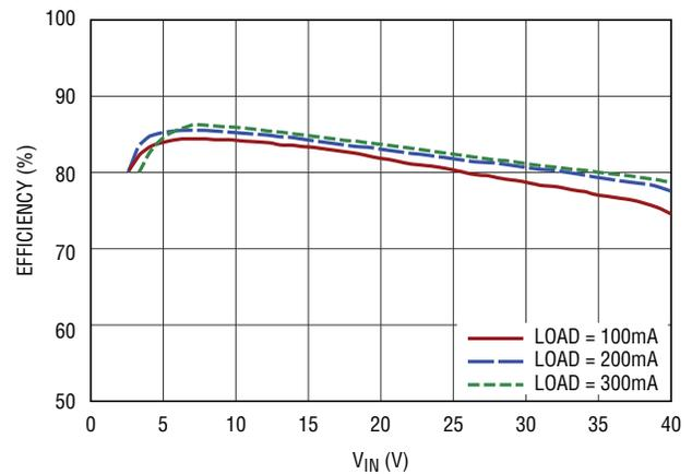
Figure 2. DC1687B Efficiency in Burst Mode Operation
