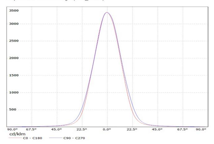
Luminaire: LEDIL OY FCN11466\_LO1-M2 (Osram Golden Dragon +) Efficiency=95% Lamps: 1 x Osram Golden Dragon (66lm@250mA)
