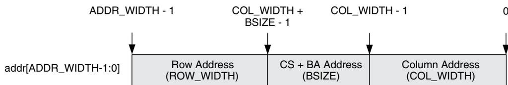
ADDR\_WIDTH is calculated by the sum of COL\_WIDTH, ROW\_WIDTH and BSIZE. BSIZE is determined by the sum of the BANK\_WIDTH and CS\_WIDTH. For LPDDR3 devices, the bank address size is always 3. Since the number of chip select is 1, the chip select address size becomes 0. An example of a typical address mapping is shown in [Table 2-4](#) and [Figure 2-8](#).
