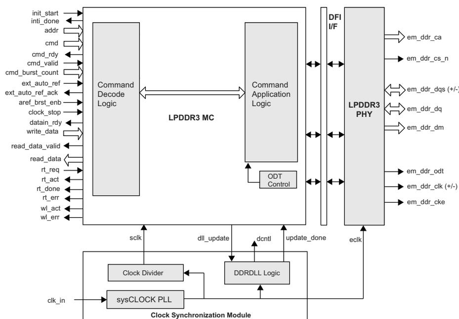
The LPDDR3 memory controller consists of three sub modules: Memory Controller (MC) module, Physical Interface (PHY) module and Clock Synchronization Module (CSM). This section briefly describes the operation of each of these modules.
