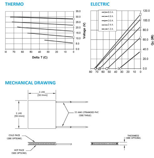
Ceramic material 96% Alumina ceramics Solder construction: 138°C BiSn
