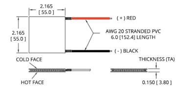
Ceramic Material: Alumina (Al<sub>2</sub>O<sub>3</sub>) Solder Construction: 138°C, Bismuth Tin (BiSn)
