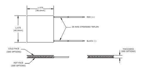
Ceramic Material: Alumina (Al<sub>2</sub>O<sub>2</sub>)
