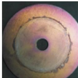
Little to no weight loss on metal coupon; less than 0.25%. Acceptable in all environments.
