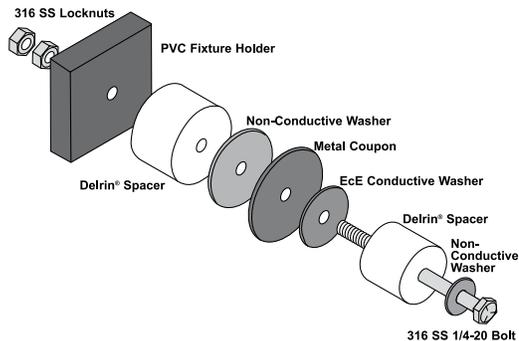
FIGURE 2. CONDUCTIVE WASHER
