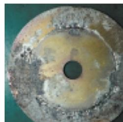
Extreme amount of weight loss on metal coupon; greater than 1.25%. Not recommended in any environments.
