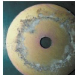
Substantial amount of weight loss on metal coupon; between 0.50% and 1.25%. Not acceptable in corrosive environments; for less corrosive applications consult with Laird applications engineer.
