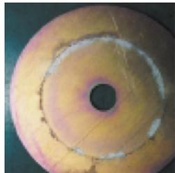
Moderate amount of weight loss on metal coupon; between 0.25% and 0.50%. May not be acceptable in very corrosive environments.
