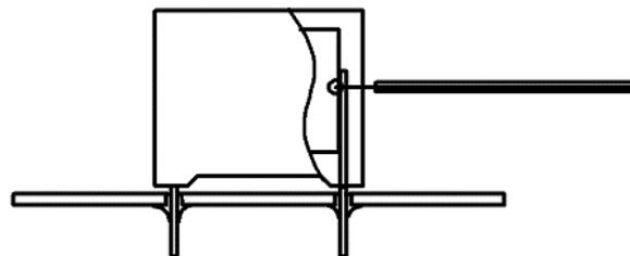
*Temperature monitored inside the capacitor.*
