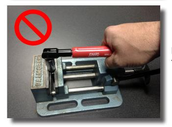
**Do not** hold the wrench to close to the bottom of the tool
