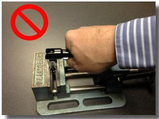
**Do not** hold the wrench to close to the top of the tool
