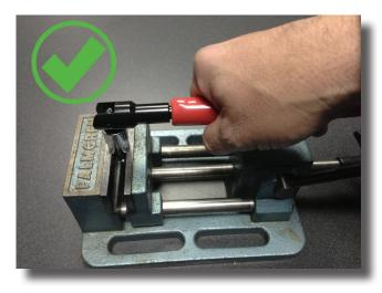
For the best most accurate results the torque wrench should be held using a full hand grip centered on handle
