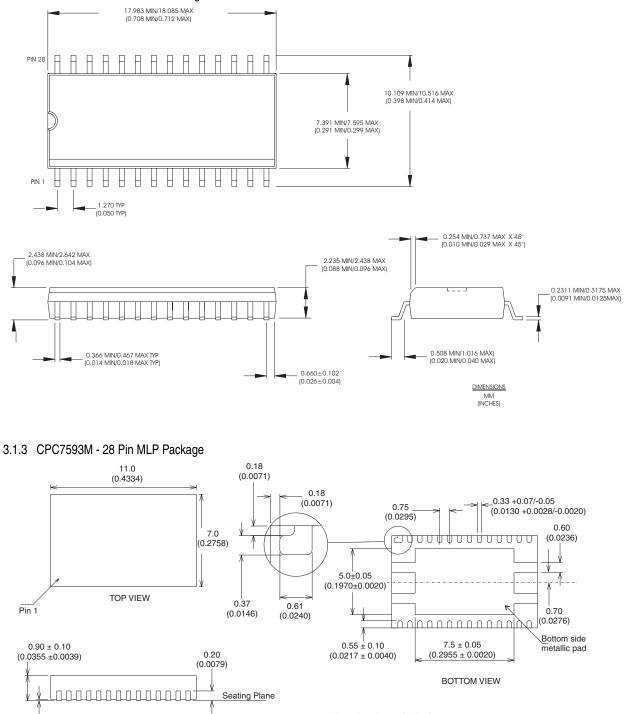
Dimensions in mm (inches) Dimensions and tolerances conform to ANSI Y14.5M-1994
