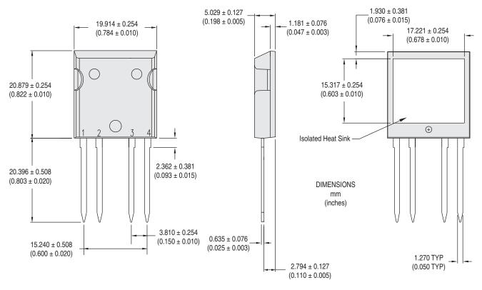
NOTE: Back-side heat sink meets 2500V<sub>rms</sub> isolation to the pins.
