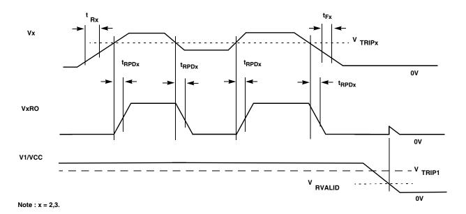
FIGURE 32. V2, V3 TIMING DIAGRAM
