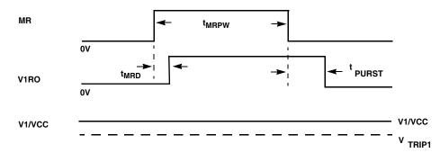
FIGURE 31. MANUAL RESET TIMING DIAGRAM
