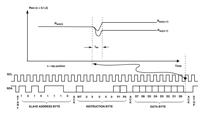
FIGURE 34. DCP "WIPER POSITION" TIMING
