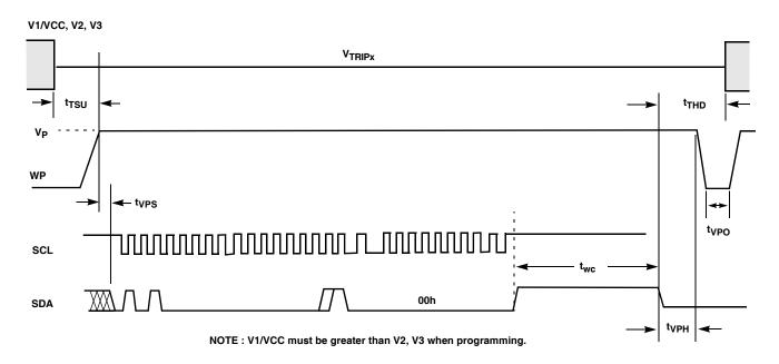
FIGURE 33. V<sub>TRIPX</sub> PROGRAMMING TIMING DIAGRAM (X = 1,2,3)
