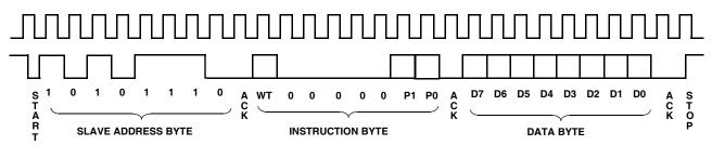
FIGURE 9. DCP WRITE COMMAND SEQUENCE
