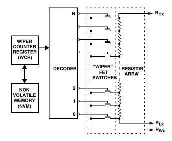
FIGURE 6. DCP INTERNAL STRUCTURE
