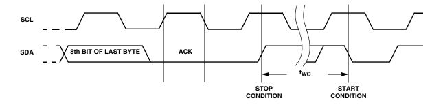
FIGURE 29. WRITE CYCLE TIMING
