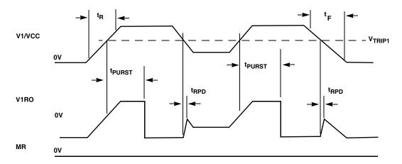
FIGURE 30. POWER-UP AND POWER-DOWN TIMING
