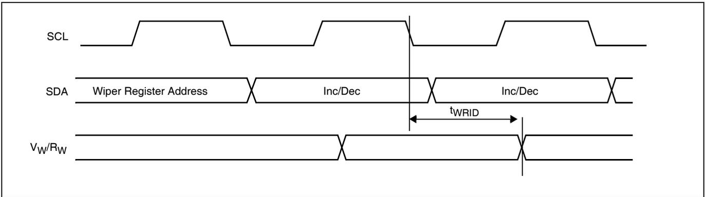
**Write Protect and Device Address Pins Timing**
