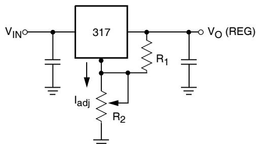
$$V_O (REG) = 1.25V (1 + R_2/R_1) + I_{adj} R_2$$
