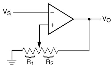
$$V_{UL} = \{R_1/(R_1 + R_2)\} V_O(max)$$
