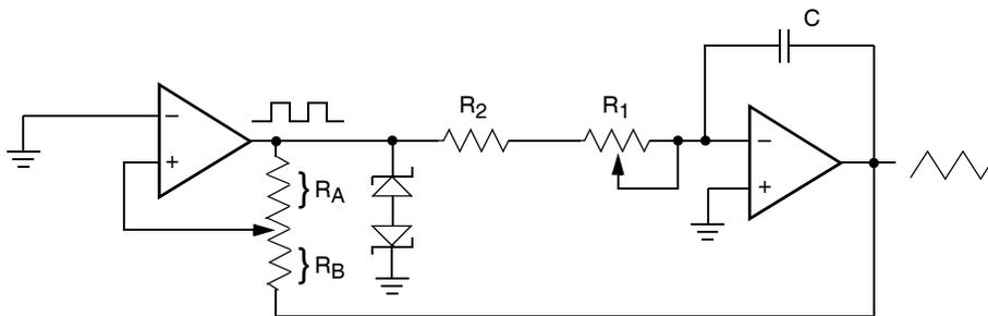
$$\text{frequency} \propto R_1, R_2, C$$
