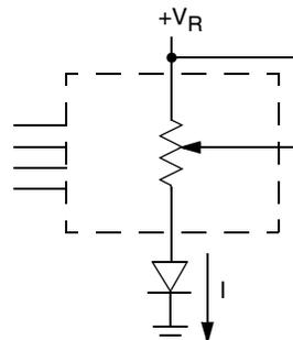
Two terminal Variable Resistor;
