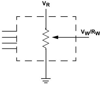
FIGURE 13. THREE TERMINAL POTENTIOMETER; VARIABLE VOLTAGE DIVIDER
