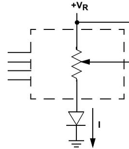
FIGURE 14. TWO TERMINAL VARIABLE RESISTOR; VARIABLE CURRENT
