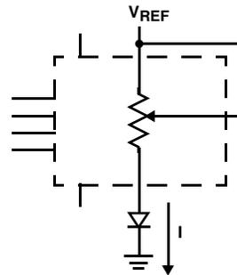
TWO TERMINAL VARIABLE RESISTOR;
