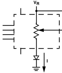
Two terminal variable resistor;
