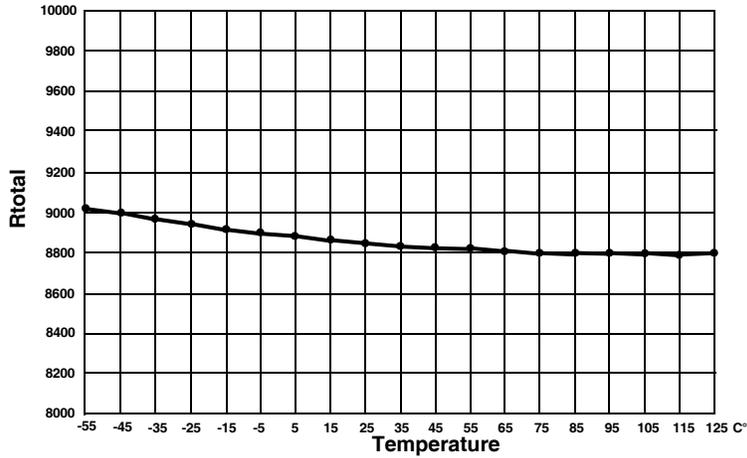
**Typical Total Resistance Temperature Coefficient**
