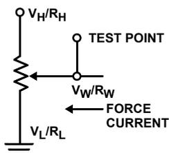
FIGURE 2. TEST CIRCUIT #2
