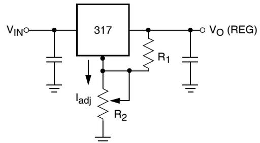
$$V_O (\text{REG}) = 1.25V (1 + R_2/R_1) + I_{adj} R_2$$
