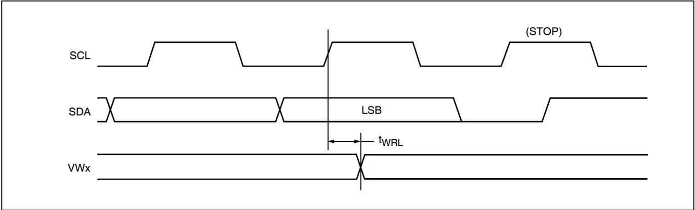
**Write Protect and Device Address Pins Timing**
