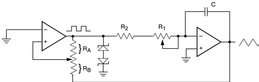
$$\text{frequency} \propto R_1, R_2, C$$
