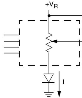
Two terminal Variable Resistor;
