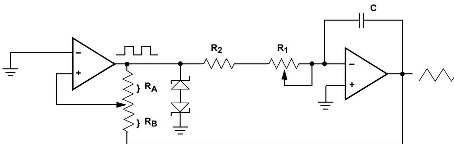
$$\text{frequency} \propto R_1, R_2, C$$
