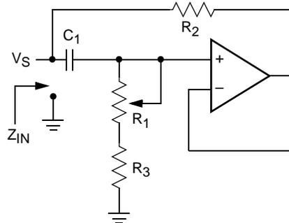
$$Z_{IN} = R_2 + s R_2 (R_1 + R_3) \quad C_1 = R_2 + s Leq$$
