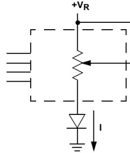
Two-terminal Variable Resistor;
