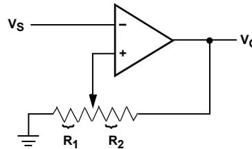
$$V_{UL} = \{R_1/(R_1 + R_2)\} V_O(\text{max})$$
