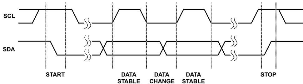
FIGURE 2. VALID DATA CHANGES, START, AND STOP CONDITIONS
