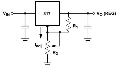
$$V_O (\text{REG}) = 1.25V (1 + R_2/R_1) + I_{adj} R_2$$
