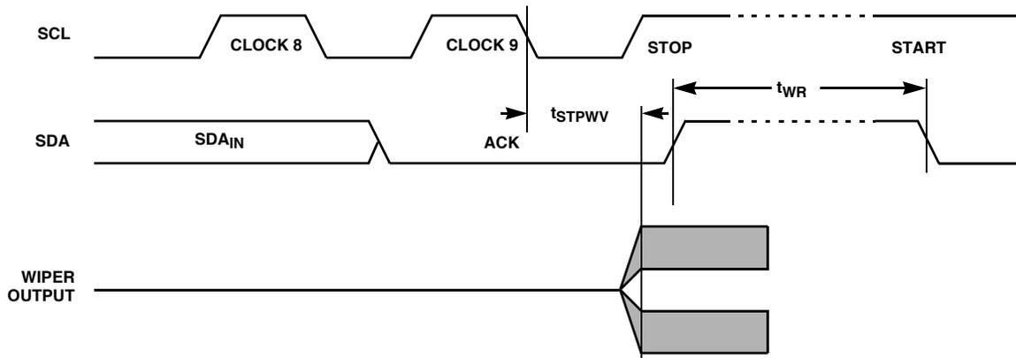
FIGURE 13. WRITE CYCLE AND WIPER RESPONSE TIMING
