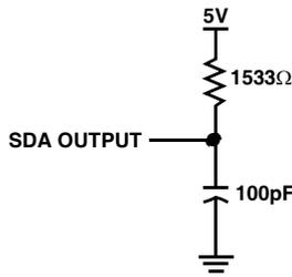
Guidelines for Calculating Typical Values of Bus Pull-Up Resistors
