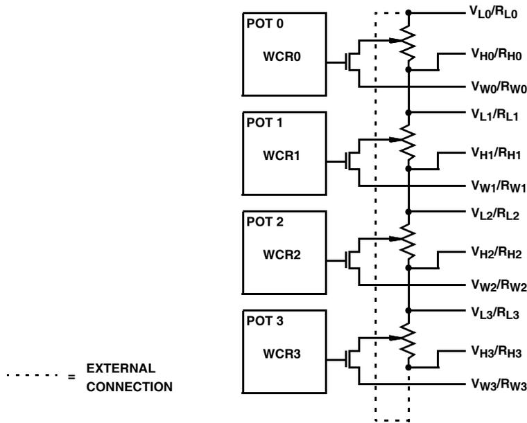
FIGURE 9. CASCADING ARRAYS
