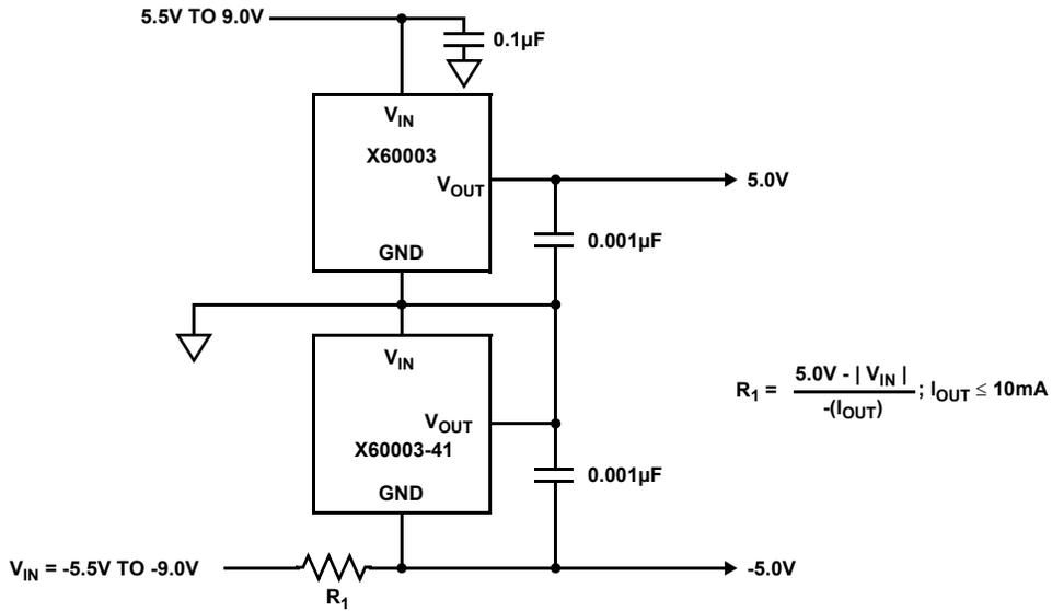
FIGURE 37. ±5.0V DUAL OUTPUT, HIGH ACCURACY REFERENCE
