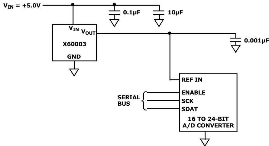
FIGURE 2. TYPICAL APPLICATION PRECISION 16 TO 24-BIT A/D CONVERTER
