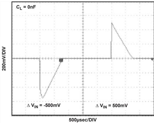
FIGURE 8. LINE TRANSIENT RESPONSE, NO CAPACITIVE LOAD
