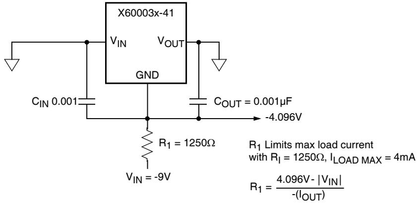
4.096V Full Scale Low-Drift 10-bit Adjustable Voltage Source
