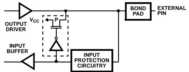
FIGURE 7. BUS HOLD CIRCUITRY PINS 26-32 AND 34
