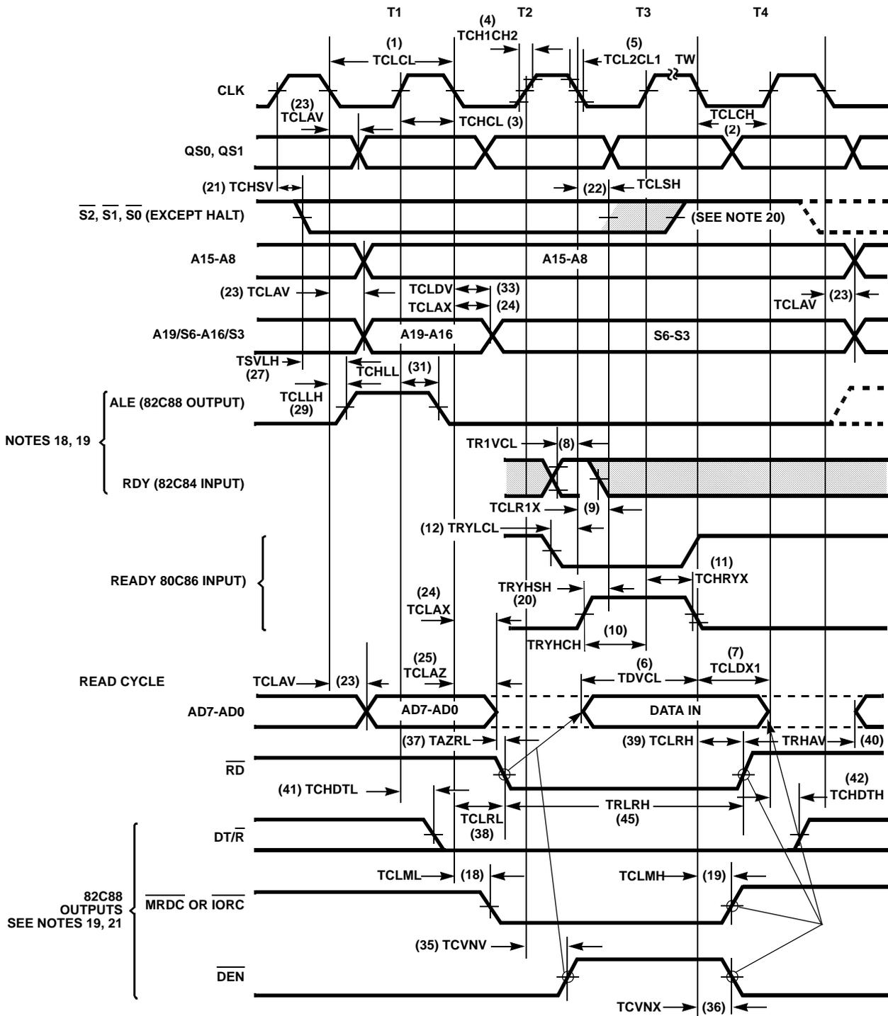
FIGURE 12. BUS TIMING - MAXIMUM MODE (USING 82C88)
