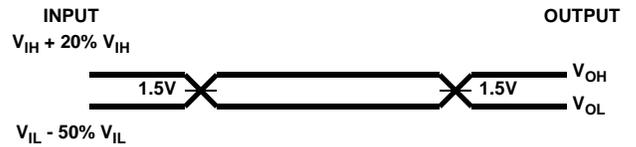
AC Testing: All input signals (other than CLK) must switch between  $V_{IL-MAX} - 50\% V_{IL}$  and  $V_{IH-MIN} + 20\% V_{IH}$ . CLK must switch between 0.4V and  $V_{CC} - 0.4V$ . Input rise and fall times are driven at 1ns/V.
