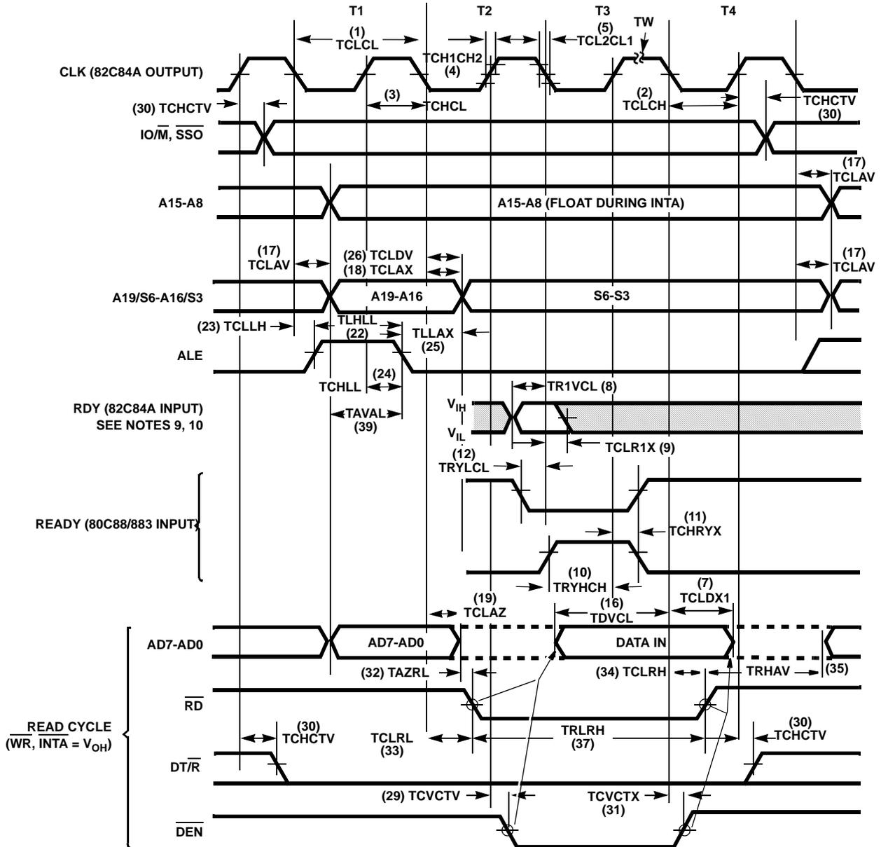
FIGURE 10. BUS TIMING - MINIMUM MODE SYSTEM
