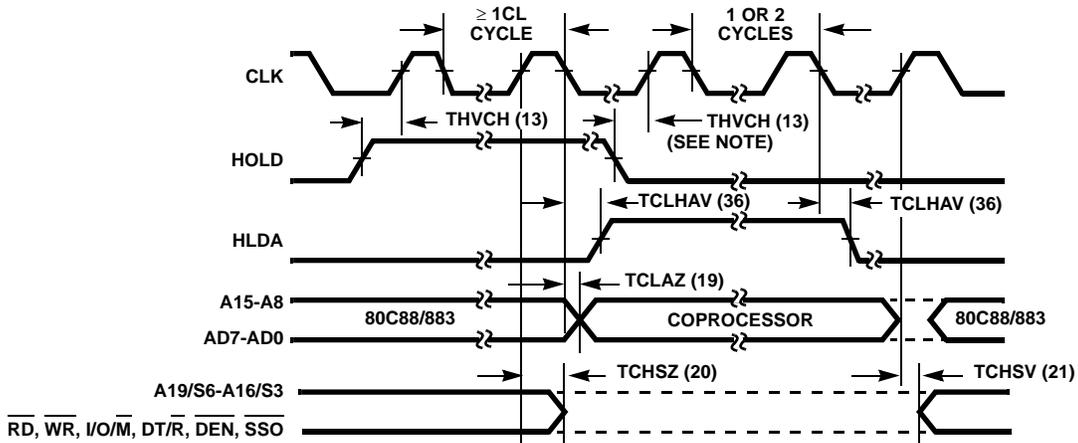
FIGURE 15. HOLD/HOLD ACKNOWLEDGE TIMING (MINIMUM MODE ONLY)
