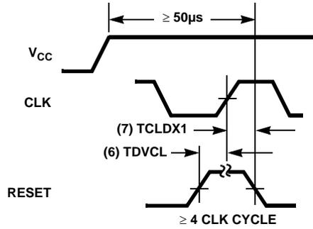
FIGURE 18. RESET TIMING
