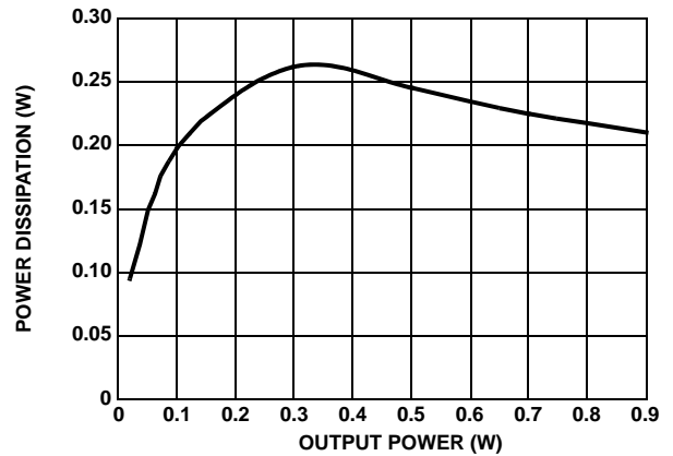
FIGURE 6. POWER DISSIPATION vs OUTPUT POWER
