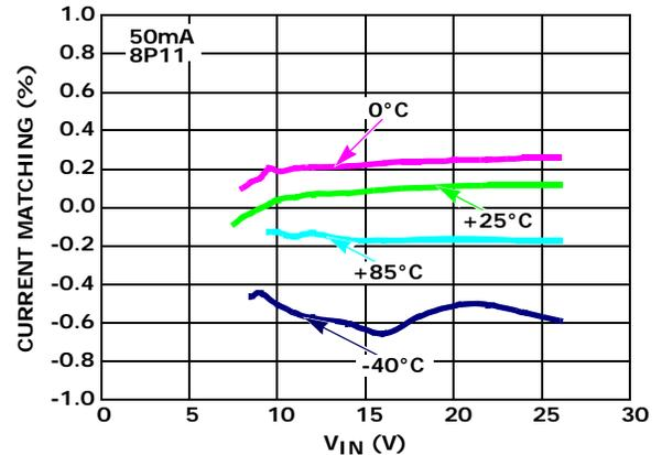
FIGURE 8. CURRENT MATCHING vs  $V_{IN}$  vs TEMPERATURE
