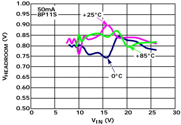
FIGURE 11.  $V_{HEADROOM}$  vs  $V_{IN}$  vs TEMPERATURE AT 50mA
