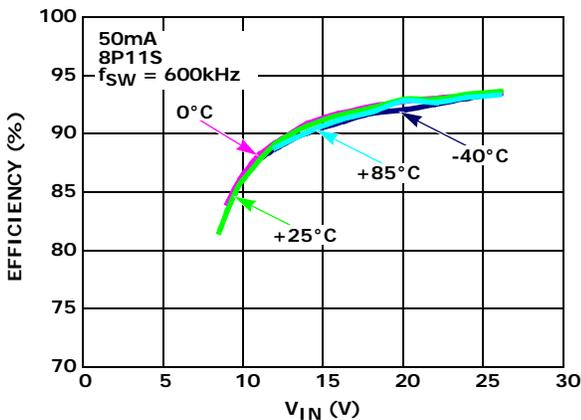
FIGURE 3. EFFICIENCY vs  $V_{IN}$  vs TEMPERATURE AT 50mA
