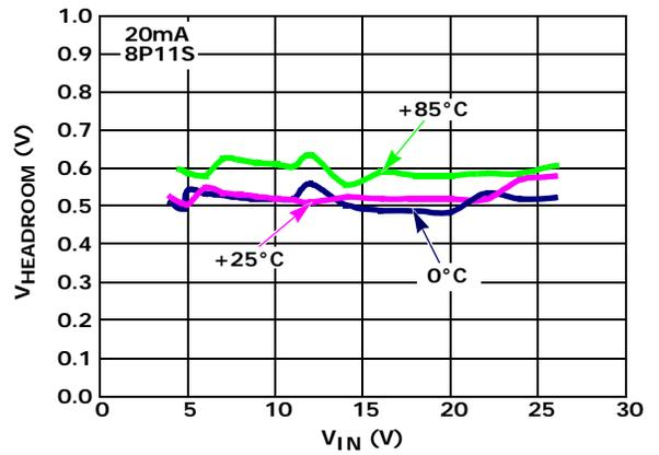
FIGURE 12.  $V_{HEADROOM}$  vs  $V_{IN}$  vs TEMPERATURE AT 20mA
