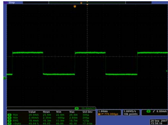
FIGURE 15. I_{LED} AT 50% PWM DIMMING
