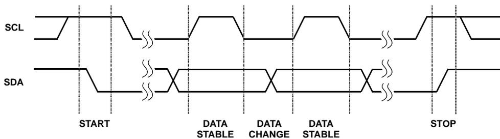
FIGURE 15. VALID DATA CHANGES, START, AND STOP CONDITIONS
