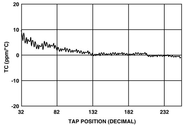
FIGURE 10. TC FOR VOLTAGE DIVIDER MODE IN ppm
