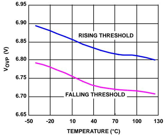
FIGURE 13. INPUT OVERVOLTAGE PROTECTION THRESHOLDS vs TEMPERATURE
