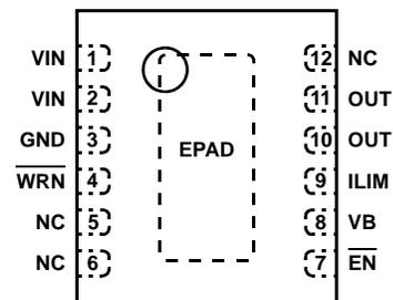
NOTE: EPAD must be electrically connected to the GND pin.
