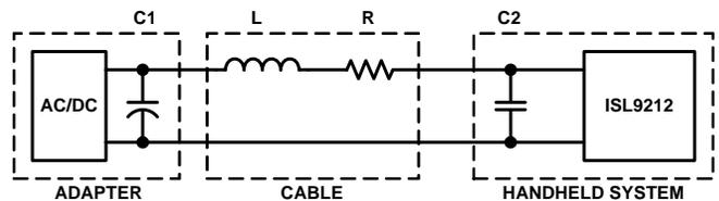
FIGURE 25. EQUIVALENT CIRCUIT FOR THE ISL9212 INPUT
