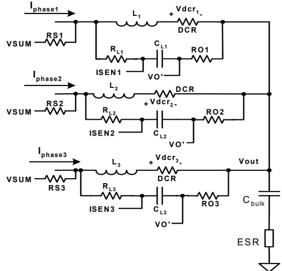
phase and one RS resistor can replace the RS resistors of each phase. The total DCR drop due to load current can be replaced by a DC source, the value of which is given by Equation 8.
