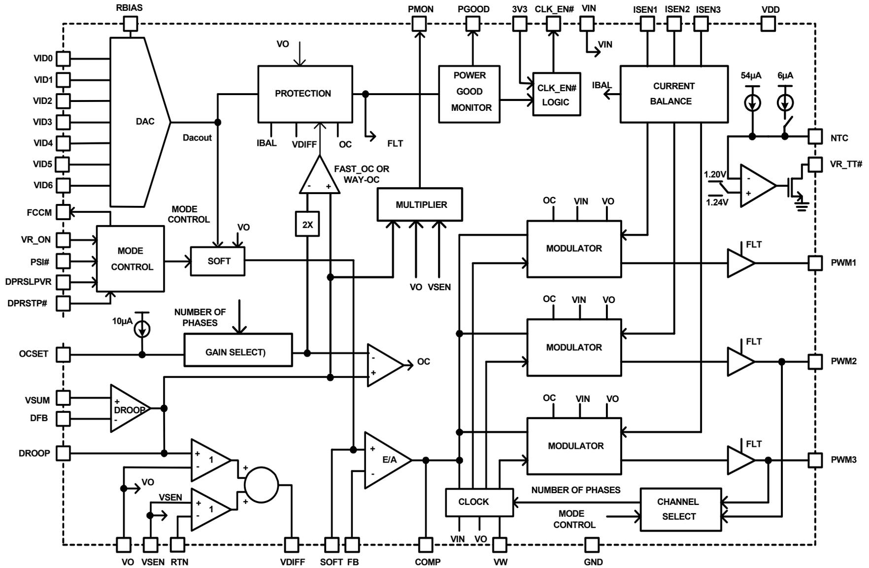
FIGURE 41. SIMPLIFIED BLOCK DIAGRAM
