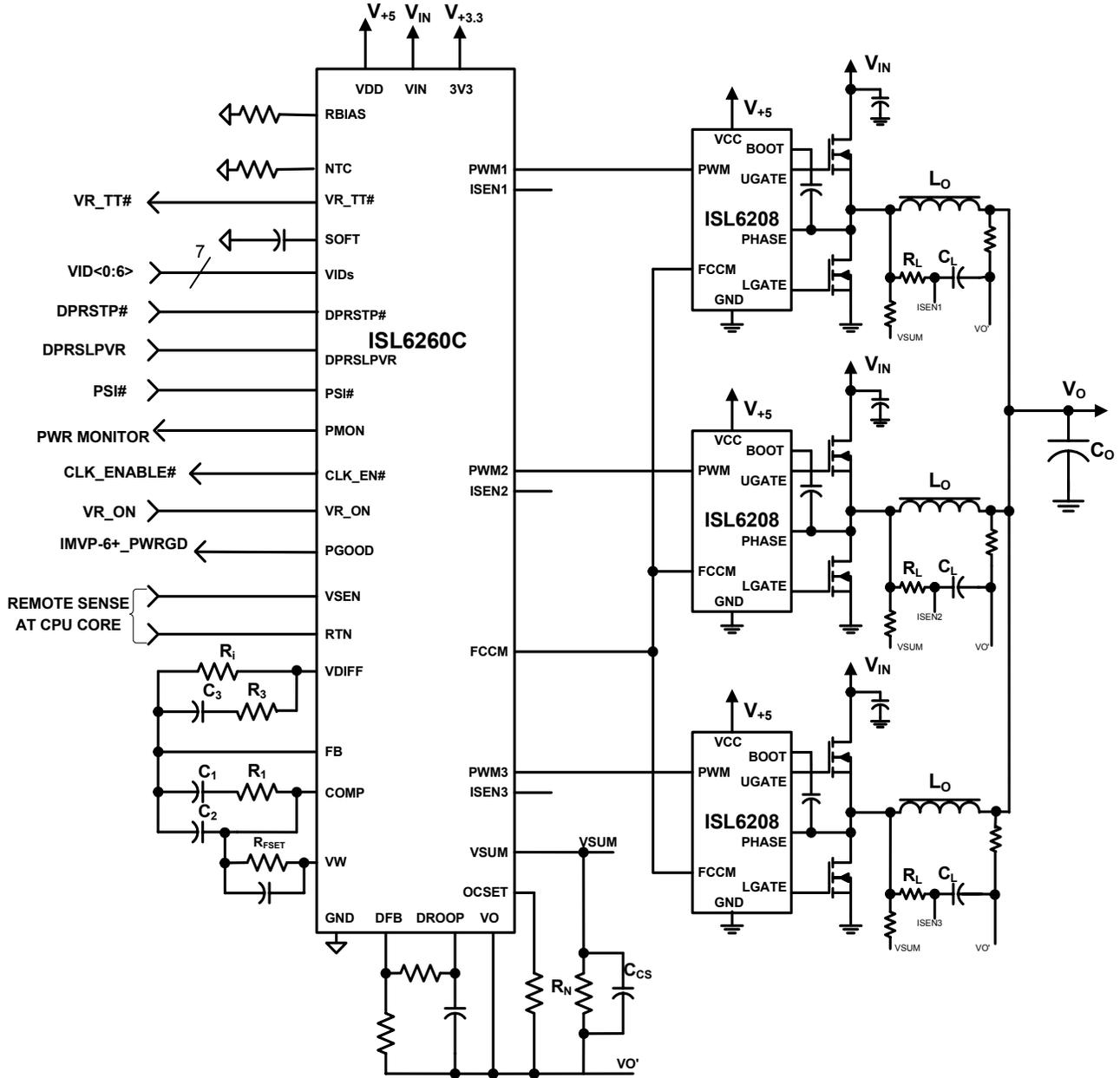
FIGURE 39. TYPICAL APPLICATION CIRCUIT FOR DCR SENSING
