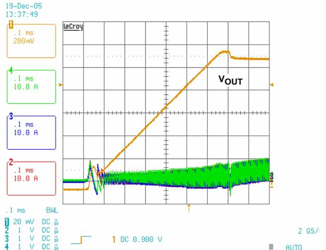
FIGURE 16. SOFT-START INRUSH CURRENT,  $V_{IN} = 8V$
