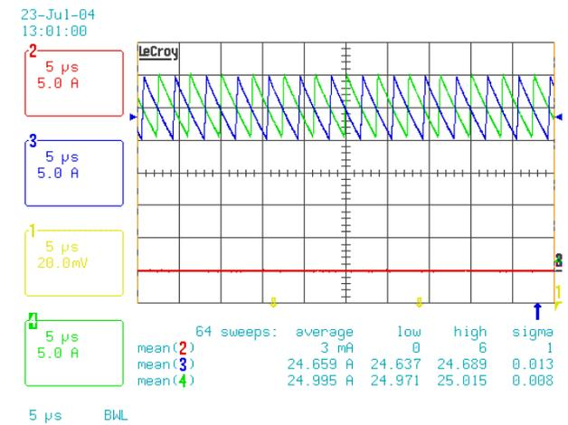
FIGURE 18. 2 PHASE CURRENT BALANCE, FULL LOAD = 50A
