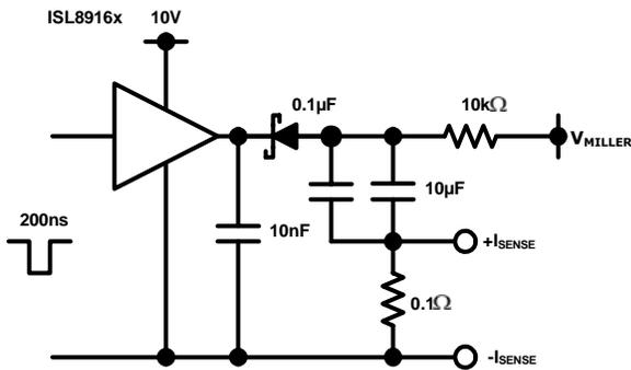
FIGURE 5. MILLER PLATEAU SINK CURRENT TEST CIRCUIT
