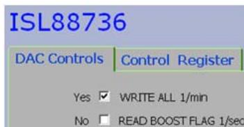
FIGURE 9. ENABLE WRITING CHARGE CURRENT REGISTER EVERY 60 SECONDS or READ THE BOOST FLAG EVERY 1 SECOND
