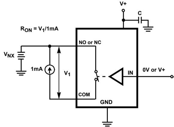
FIGURE 5.  $R_{ON}$  TEST CIRCUIT
