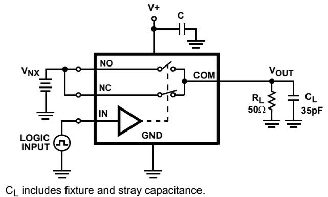
$C_L$  includes fixture and stray capacitance.
