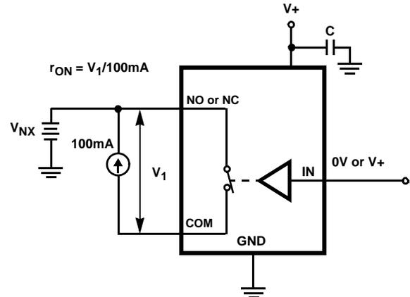
FIGURE 5.  $r_{ON}$  TEST CIRCUIT
