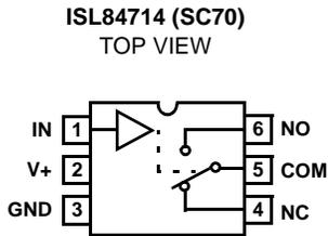
Note: Switches Shown for Logic "0" Input.
