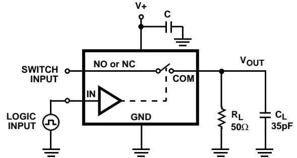
NOTE: REPEAT TEST FOR ALL SWITCHES.  $C_L$  INCLUDES FIXTURE AND STRAY CAPACITANCE.
