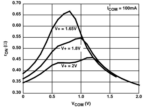
FIGURE 11. ON-RESISTANCE vs SUPPLY VOLTAGE vs SWITCH VOLTAGE
