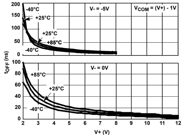
FIGURE 14. INHIBIT TURN-OFF TIME vs SUPPLY VOLTAGE
