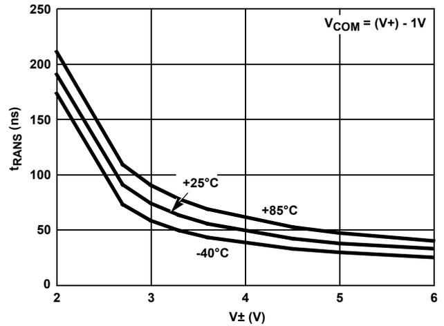
FIGURE 16. ADDRESS TRANS TIME vs DUAL SUPPLY VOLTAGE
