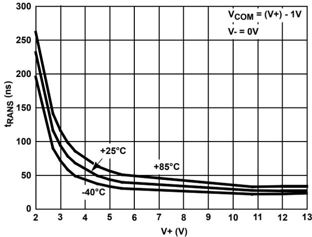
FIGURE 15. ADDRESS TRANS TIME vs SINGLE SUPPLY VOLTAGE
