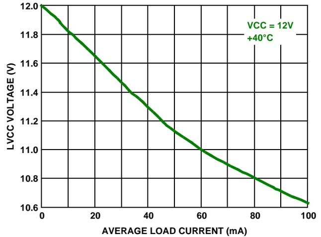
FIGURE 3. TYPICAL LVCC VARIATION WITH LOAD (CCM)
