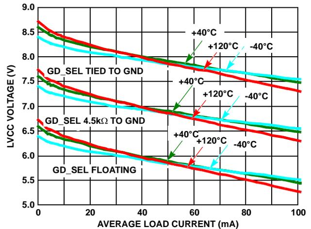
FIGURE 4. TYPICAL LVCC VARIATION WITH LOAD (DEM)
