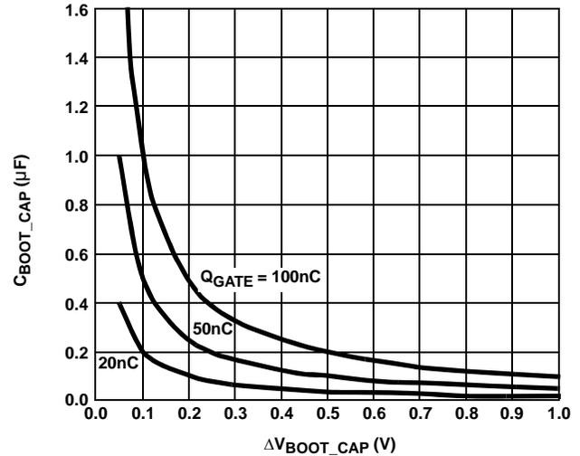
FIGURE 2. BOOTSTRAP CAPACITANCE vs BOOT RIPPLE VOLTAGE
