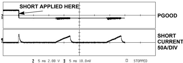
**HICCUP MODE. SUPPLY POWERED BY ATX SUPPLY**
