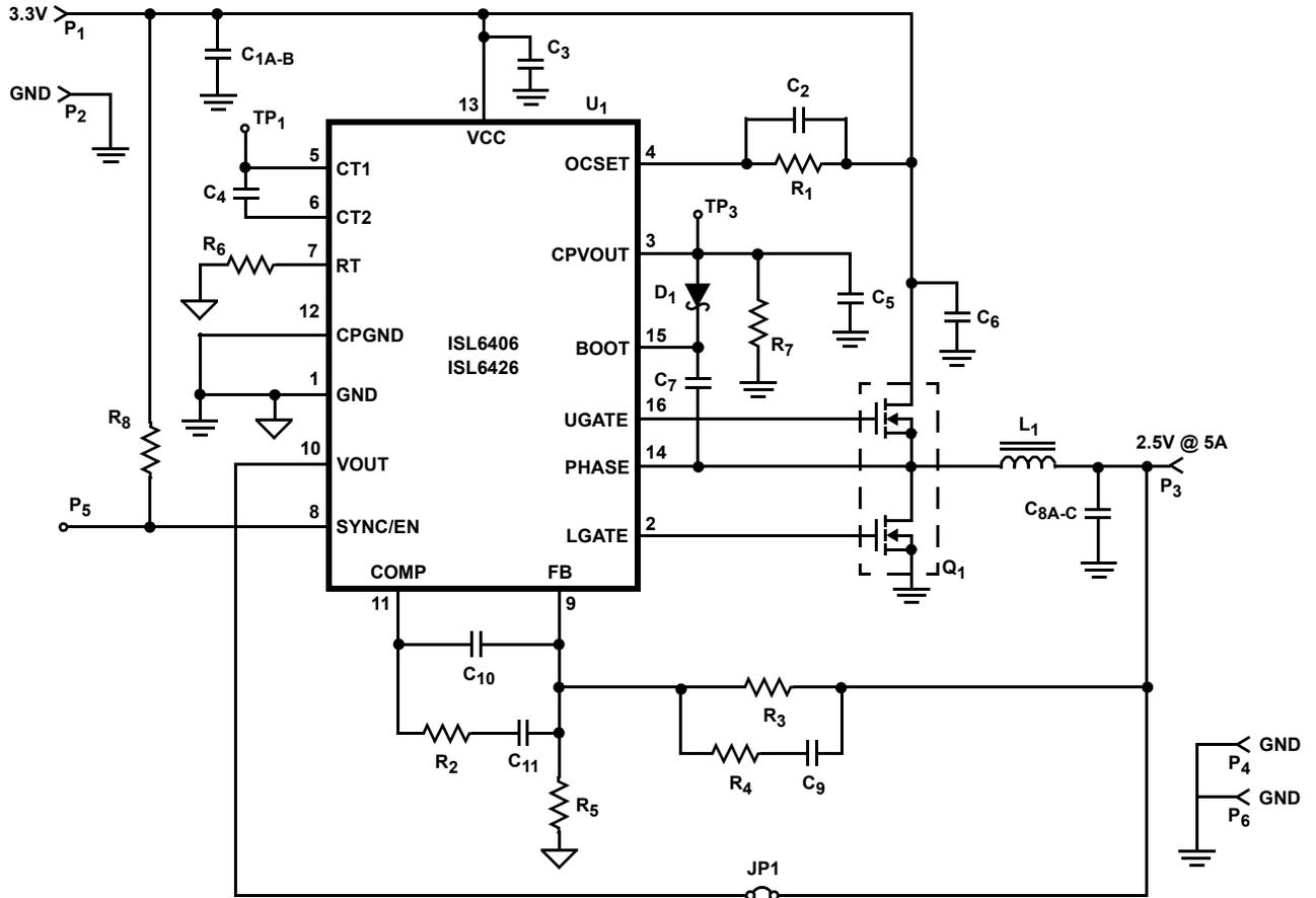
NOTE: Remove R3, R4, C9, and R5 from the board and close JP1 for ISL6426 evaluation.
