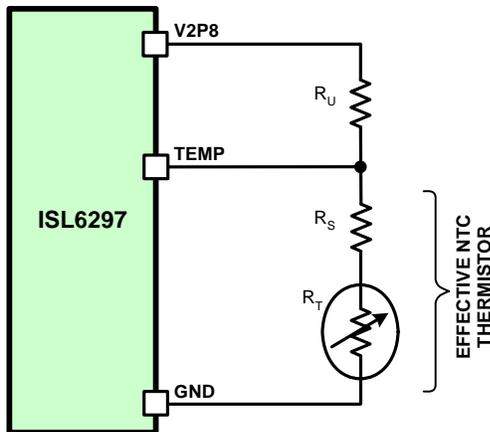
FIGURE 12. EFFECTIVE NTC THERMISTOR CIRCUIT
