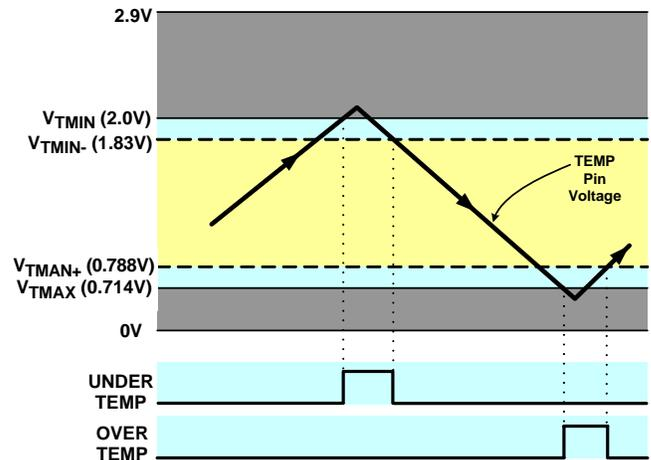
FIGURE 11. CRITICAL VOLTAGE LEVELS FOR TEMP PIN
