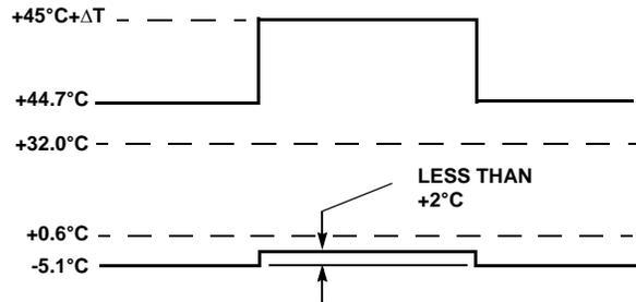
**FIGURE 13. BOARD TEMPERATURE MONITORING. WHEN NOT CHARGING, THE TEMPERATURE WINDOW IS BETWEEN -5 $^{\circ}\text{C}$  AND +45 $^{\circ}\text{C}$ . ONCE THE CHARGER STARTS, THE TEMPERATURE WINDOW IS -3 $^{\circ}\text{C}$  TO +45 $^{\circ}\text{C} + \Delta T$**
