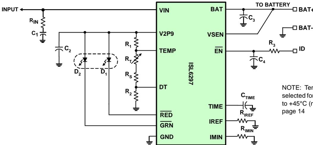
NOTE: Temperature limit components selected for a temperature Range of -5°C to +45°C (not charging) See Example, page 14
