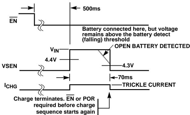
FIGURE 5. OPEN BATTERY DETECTED
