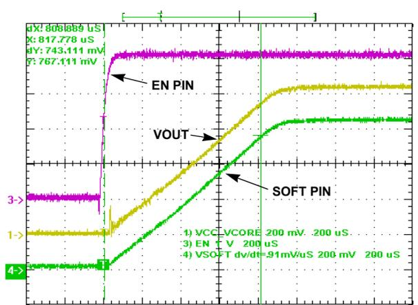
Soft-start into CCM, VIN = 4.2V, CH3 = EN pin. Vout = 0.85
