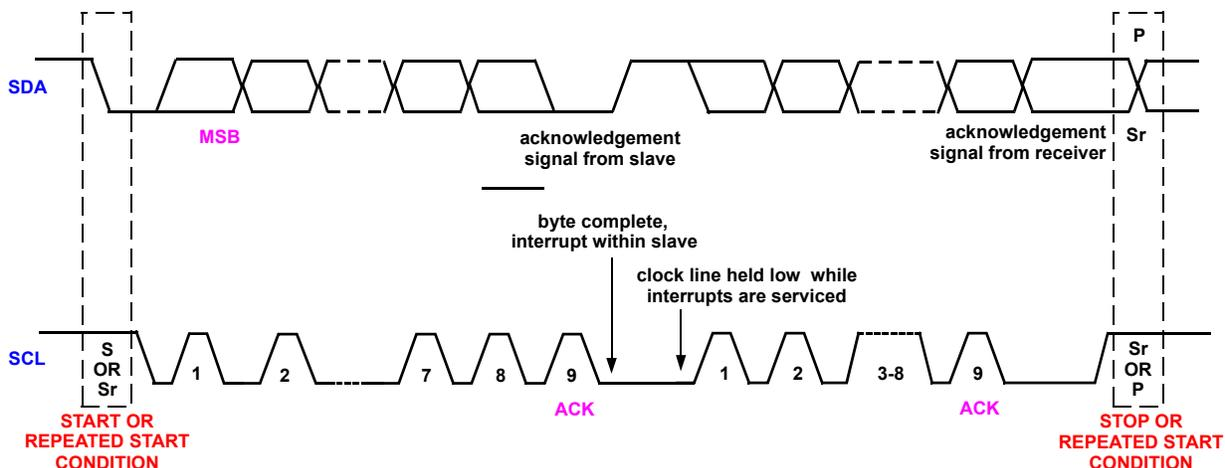
FIGURE 17. I<sup>2</sup>C DATA AND CLOCK
