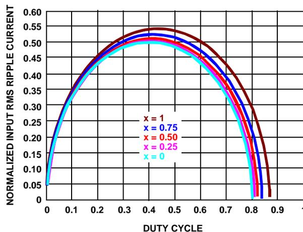
FIGURE 7. NORMALIZED RMS INPUT CURRENT FOR  $x = 0.8$
