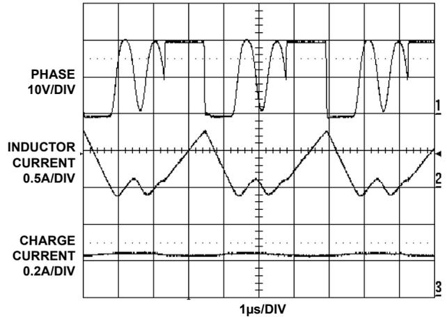
FIGURE 14. SWITCHING WAVEFORMS AT TRICKLE CHARGE MODE
