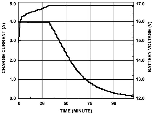
FIGURE 3. BATTERY CHARGE V-I CHARACTERISTICS
