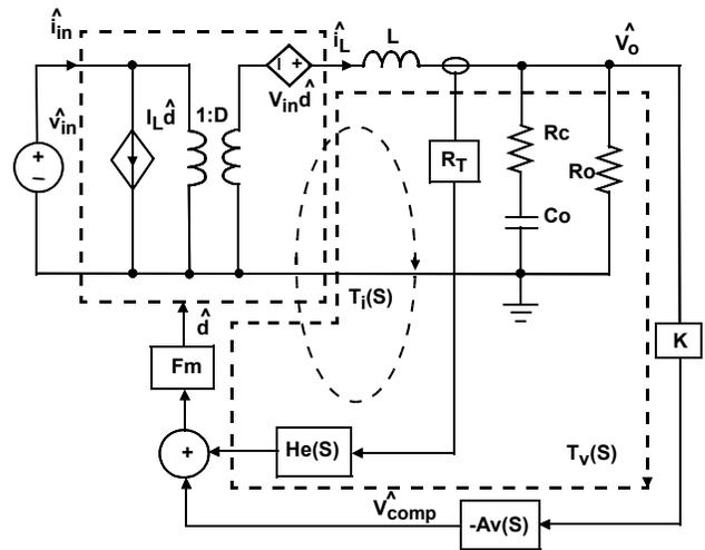
FIGURE 19. SMALL SIGNAL MODEL OF SYNCHRONOUS BUCK REGULATOR
