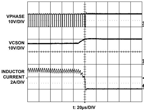
FIGURE 11. BATTERY REMOVAL
