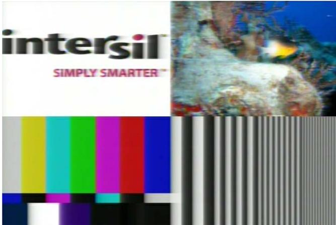
**FIGURE 5. TEST PATTERN IMAGE AFTER 2000 FEET OF UNCOMPENSATED CAT 5**
