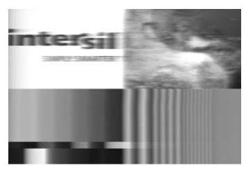
FIGURE 17. TEST PATTERN IMAGE AFTER 5200 FEET OF UNCOMPENSATED CAT 5
