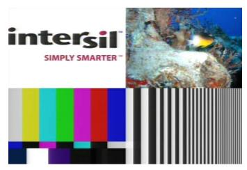
FIGURE 25. TEST PATTERN IMAGE AFTER 2000 FEET OF UNCOMPENSATED RG-59 COAX
