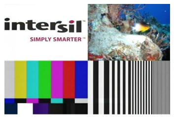
FIGURE 18. TEST PATTERN IMAGE AFTER 5200 FEET OF CAT 5
