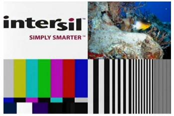
FIGURE 6. TEST PATTERN IMAGE AFTER 2000 FEET OF CAT 5
