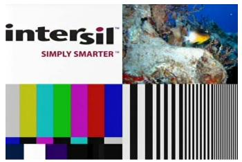
FIGURE 10. TEST PATTERN IMAGE AFTER 3000 FEET OF CAT 5
