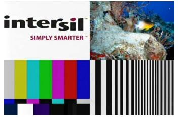
FIGURE 2. TEST PATTERN IMAGE AFTER 1000 FEET OF CAT 5
