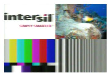
FIGURE 9. TEST PATTERN IMAGE AFTER 3000 FEET OF UNCOMPENSATED CAT 5
