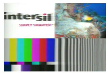
FIGURE 41. TEST PATTERN IMAGE AFTER 6000 FEET OF UNCOMPENSATED RG-59 COAX
