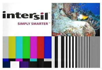
FIGURE 42. TEST PATTERN IMAGE AFTER 6000 FEET OF RG-59
