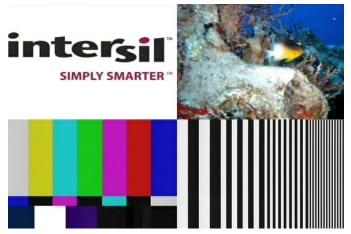
FIGURE 14. TEST PATTERN IMAGE AFTER 4000 FEET OF CAT 5
