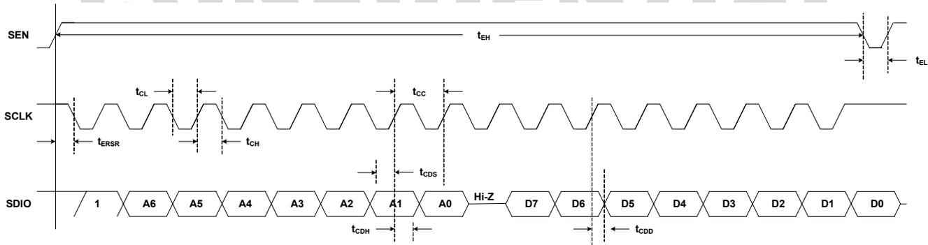
FIGURE 17. SPI SERIAL INTERFACE WRITE CYCLE TIMING DIAGRAM
