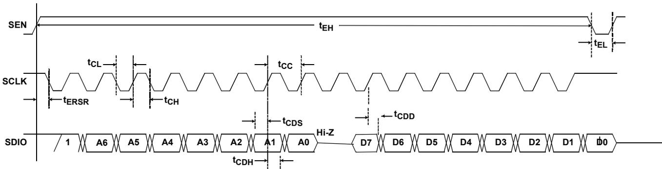
FIGURE 18. SPI SERIAL INTERFACE READ CYCLE TIMING DIAGRAM
