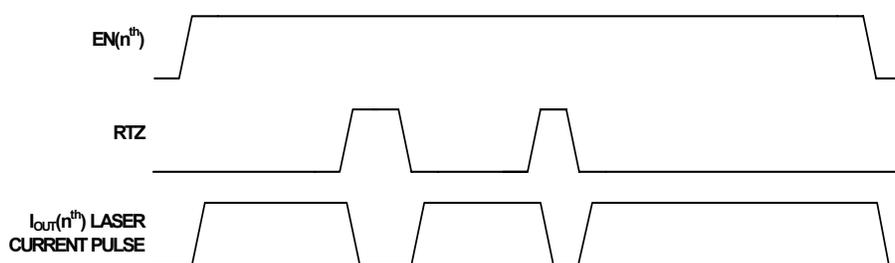
FIGURE 14. ASYNCHRONOUS RETURN-TO-ZERO MODE PULSE TIMING DIAGRAM FOR INPUT PIXEL MODE 3
