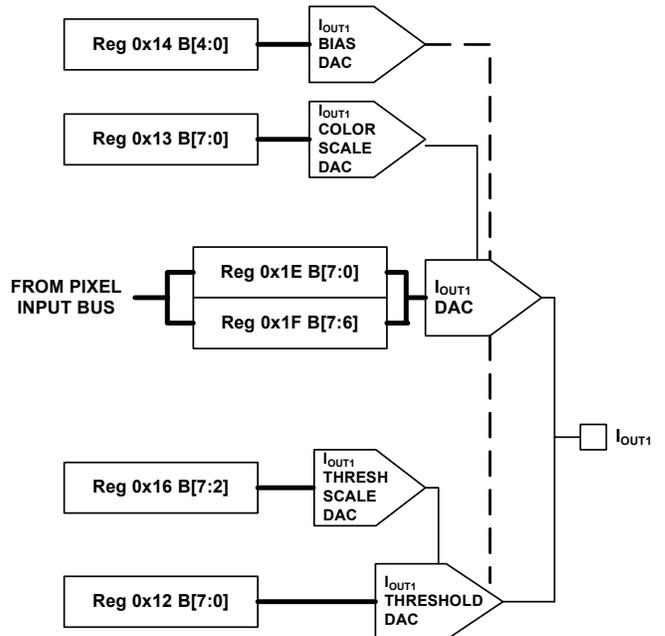
FIGURE 8. I<sub>OUT1</sub> N-MOS OUTPUT DAC BLOCK DIAGRAM
