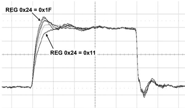
FIGURE 25.  $I_{OUT2}$  WAVEFORM AT DIFFERENT BIAS VOLTAGES
