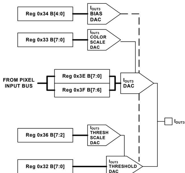
FIGURE 9. I<sub>OUT3</sub> N-MOS OUTPUT DAC BLOCK DIAGRAM
