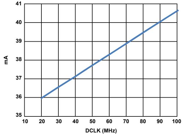
FIGURE 26. TOTAL CURRENT vs. INPUT CLOCK FREQUENCY.
