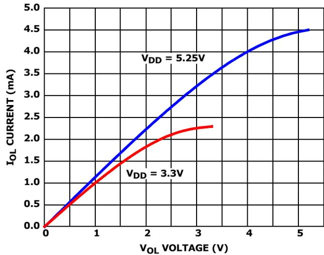
FIGURE 18.  $I_{OL}$  vs  $V_{OL}$  vs  $V_{DD}$  for  $\overline{\text{INT}}$
