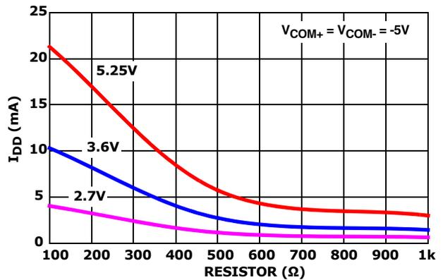
**FIGURE 7. NEGATIVE OVP I<sub>DD</sub> CURRENT vs RESISTOR VALUE vs V<sub>SUPPLY</sub>**
