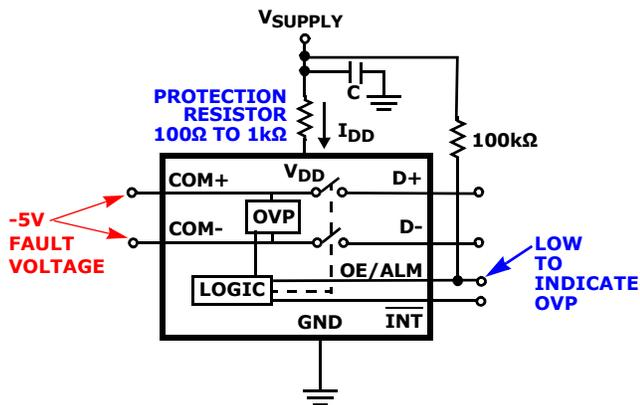
**FIGURE 6. V<sub>DD</sub> SERIES RESISTOR TO LIMIT I<sub>DD</sub> CURRENT DURING NEGATIVE OVP AND FOR ENHANCED ESD AND LATCH-UP IMMUNITY**
